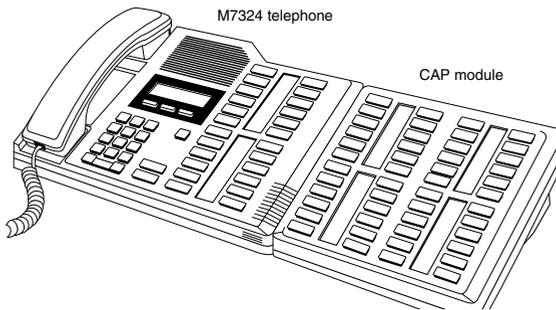
A CAP module is an add-on device that provides 48 extra memory or line buttons. You can connect one or two Norstar CAP modules to the telephone to increase the number of lines it can handle.
